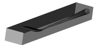
h) Vortex extent computed on mesh shown in (g) – vortex volume 0.07587\text{m}^3
